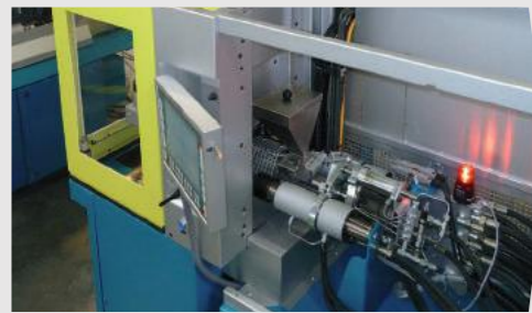
Injection unit for 2C injection moulding tightly mounted on the machine table
