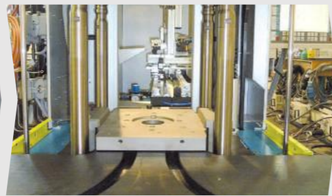
Y-table with curved tracks and integrated automation on the machine table
