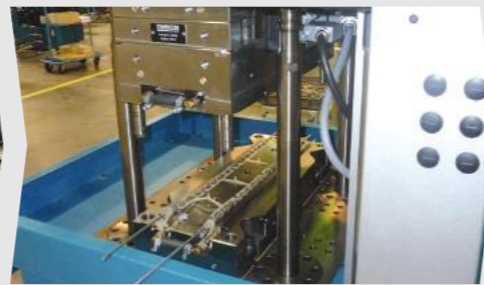
Continuous production of distance pieces of saw chains
