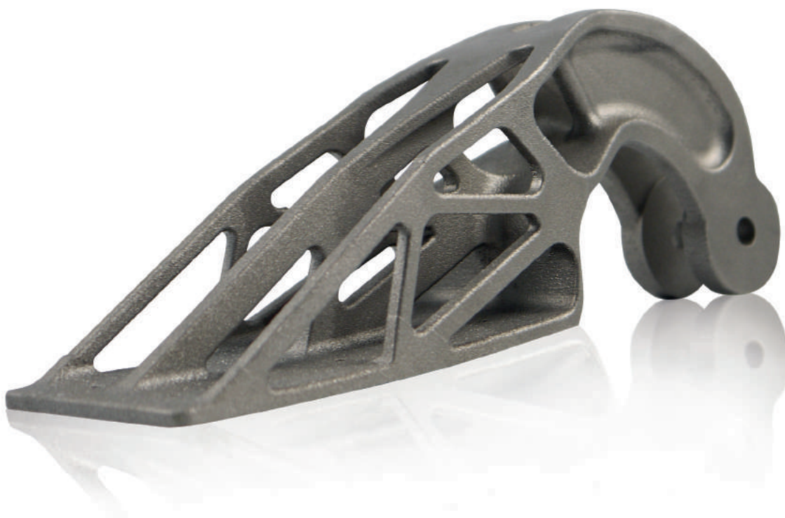
Demonstration part of a nacelle hinge bracket for an Airbus A320 with optimized topology; built in titanium by using an EOS M 290 (Source: Airbus Group Innovations).
